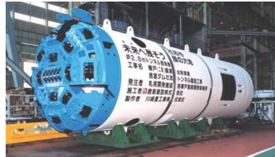
φ2.8m full shield TBM(belt conveyor discharge system)
