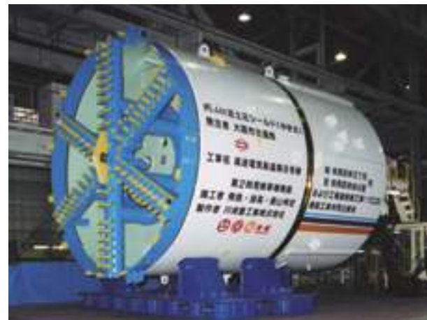
φ5.44m earth pressure balanced shield machine
