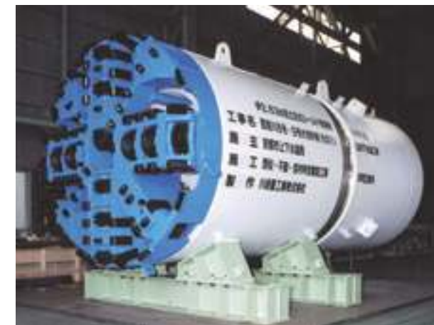
φ2.63m earth pressure balanced shield machine
