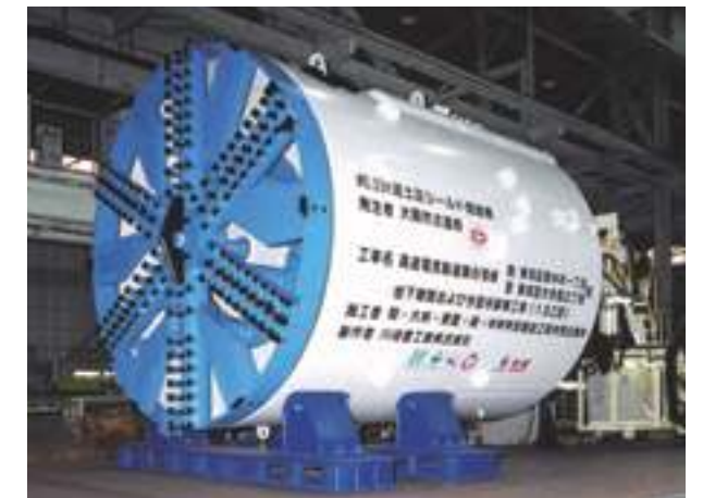
φ5.33m earth pressure balanced shield machine
