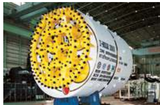
φ7.67m earth pressure balanced DPLEX shield machine
