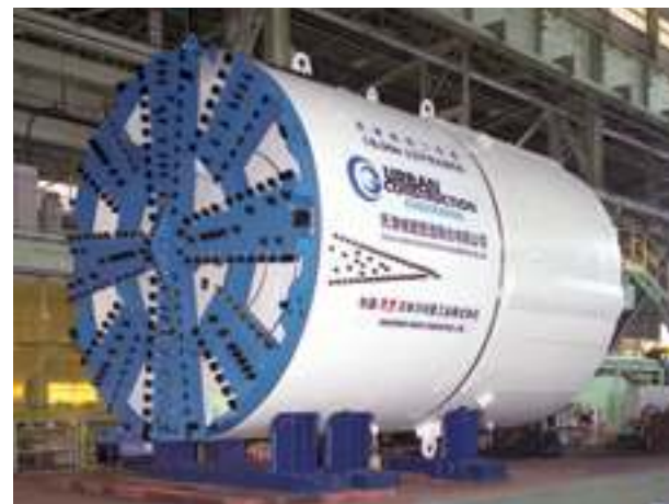
φ6.34m earth pressure balanced shield machine
