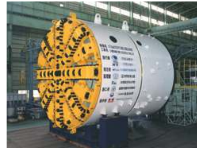
φ7.93m earth pressure balanced shield machine
