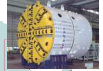
φ7.80m slurry shield machine (Soul subway No.9, Korea)
