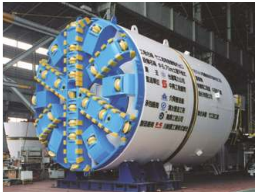
φ6.70m earth pressure balanced shield machine
