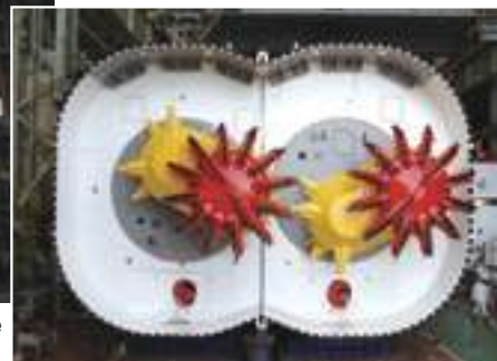
7.44m×10.64m earth pressure balanced rectangular shield machine
