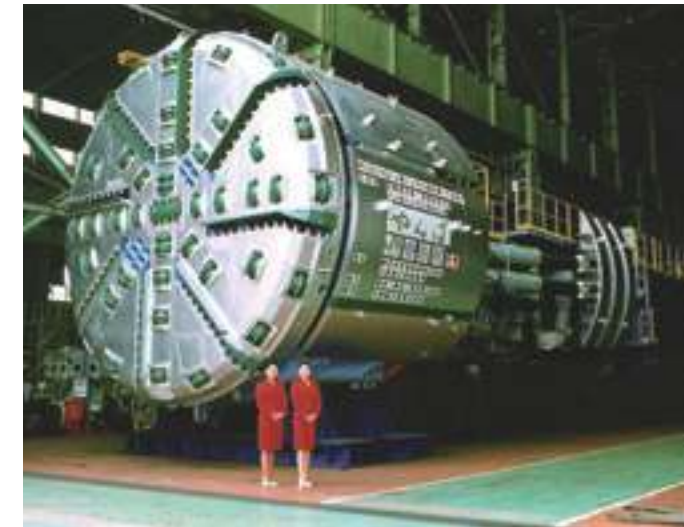
φ6.82m open gripper TBM
