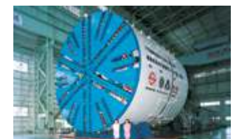
φ10.04m single shield machine (without side shields)
