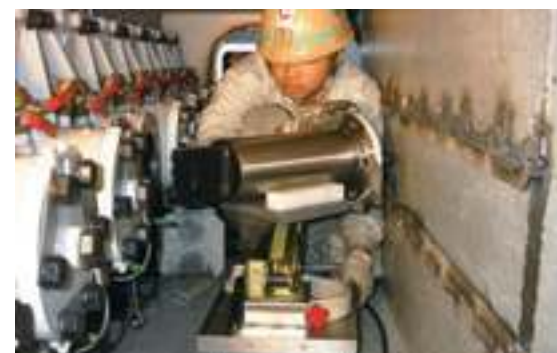
During cutter change from inside
