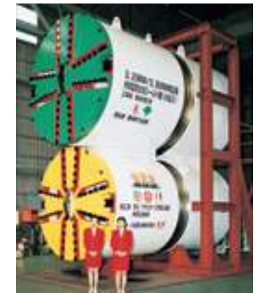
φ3.29m / φ2.89m dual-mount branching H&V shield machine
