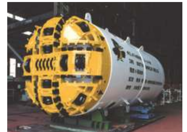
φ2.47m slurry shield machine for bedrock
