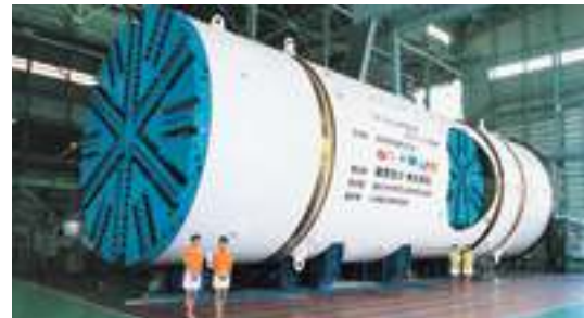
φ7.26m/φ4.24m slurry subterranean stem shield machine
