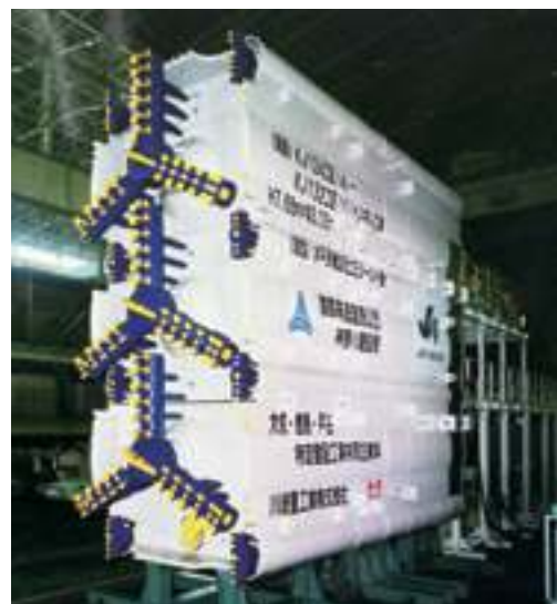
H7.86m×W3.05m multi-axial rectangular slurry shield machine
