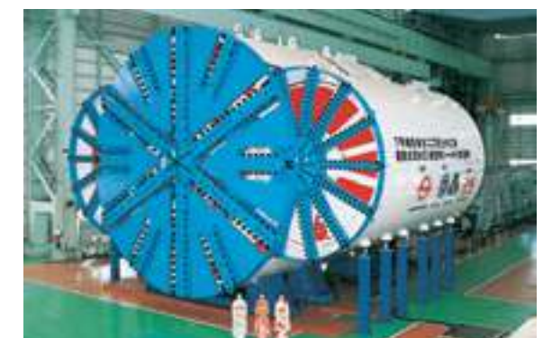
φ10.04m×15.84m three-section shield machine (with side shields attached)
