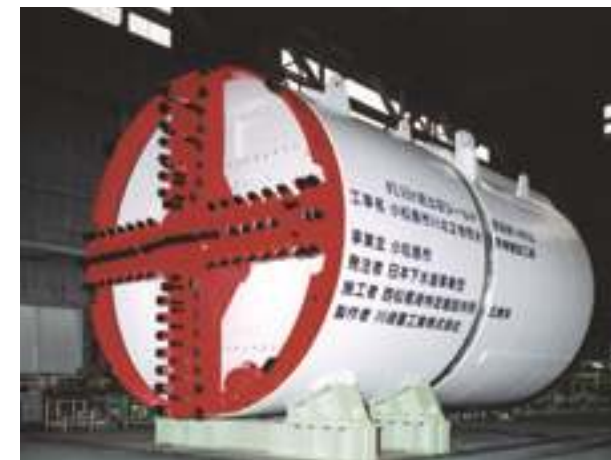
φ3.93m earth pressure balanced shield machine
