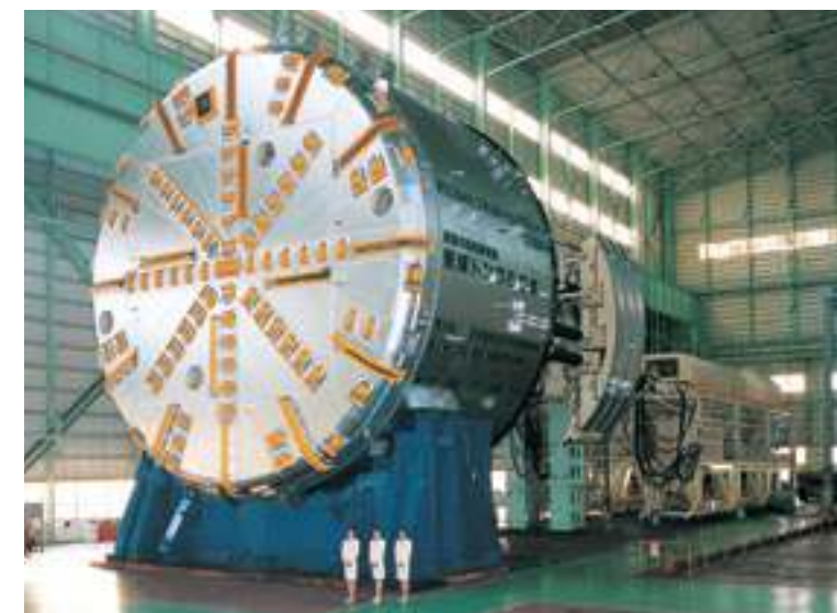
φ12.84m new open TBM
