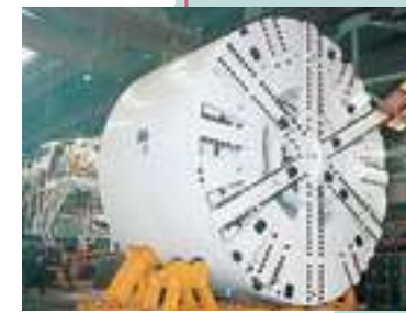
φ9.74m earth pressure balanced shield machine (Lisbon subway No. 2 Line, Portugal)
