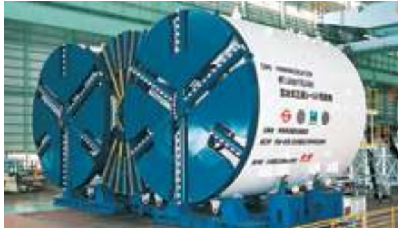
φ7.44m×16.44 slurry three-section shield machine
